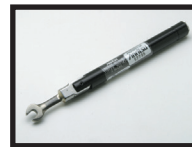
01-506, W1-7 mm Fixed break over torque wrench: 7 mm opening for W1-105x Sparkplug installation. Torque is 0.56 N*m (5 in-lbs)
